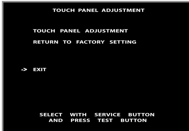
If you have an issue with the 'Touch Panel' positioning being slightly off, the following procedure should be carried out.
