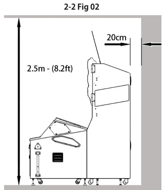
Before leaving the machine after Installation, make sure that the Castor Lift Adjusters are firmly positioned on the ground and that the machine is totally stable.
