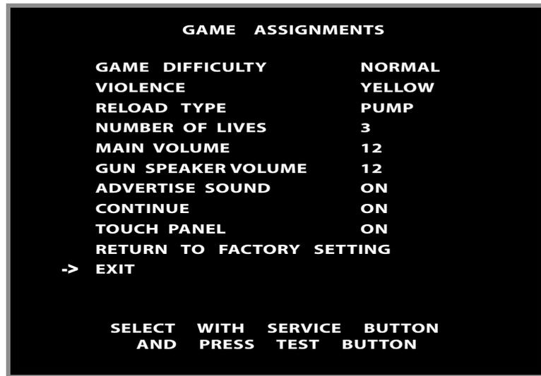
Press the **SERVICE** Button to step the Arrow around to select the function required, then press the **TEST** Button to gain entry.
